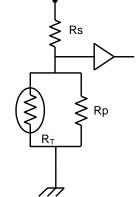
Driving Voltage Controlled by Temperature
